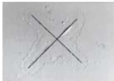
Figure 7 : Aspect of cross-scratched sample after edge creep testing (four-leaved clover)
